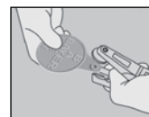
Figure 2 Slide tag under the clip of the pliers by depressing the lever.
